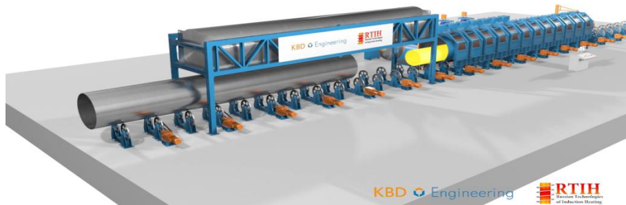
Fig.3 – Stage hardening (two separate zones: induction oscillating heating and quenching)
